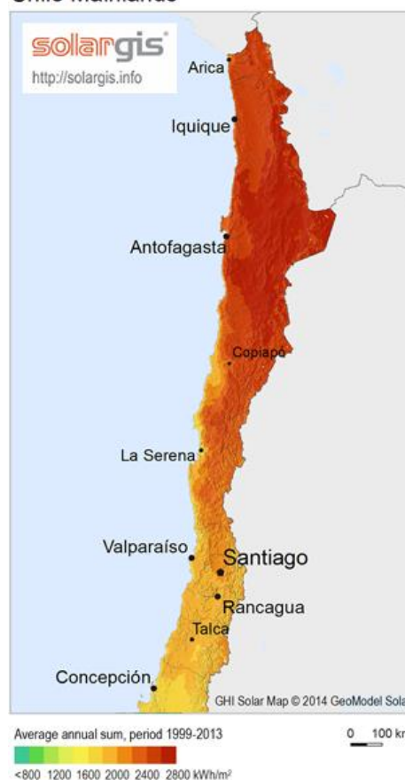
Figure 1: Yearly average GHI in the northern half of Chile. Source: SolarGIS [2]
